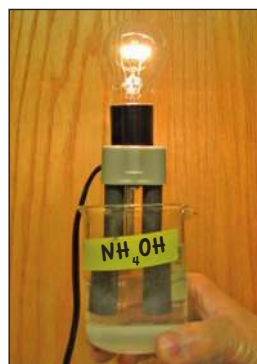
▲ Figure (20) The strong base conducts an electrical current to a larger degree than the weak base
