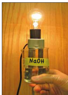
▲ Figure (20) The strong base conducts an electrical current to a larger degree than the weak base
